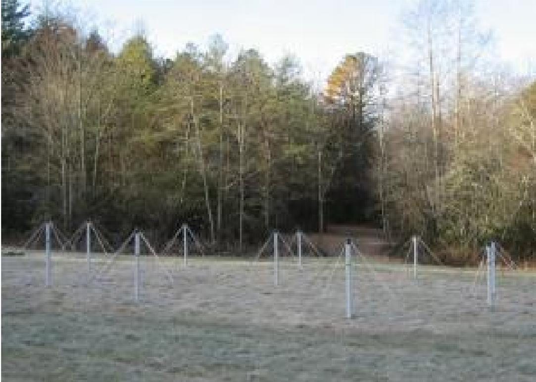
*The Eight-meter-wavelength Transient Array, being set up to search the sky for these radio pulses from explosions up to 300 light years away. (Credit: Image courtesy of John Simonetti / Virginia Tech)*
